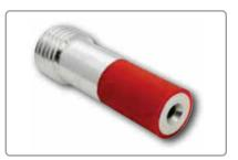
Featuring a liner made from hot-pressed boron carbide, this nozzle offers chemical and wear resistance properties, making it ideal for abrasives such as garnet, aluminium oxide and steel grit. As well as being heat and corrosion resistant, the nozzle's aluminium jacket makes it lightweight and its rubber sleeve is shock absorbent, preserving the internal liner. The nozzles are supplied with a rubber gasket.
