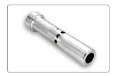
This nozzle offers a 35% larger blast pattern than a standard Venturi nozzle with only a small loss in abrasive velocity. Designed to be used on jobs where a more even dispersion of abrasive is required through a larger blast pattern. Supplied with a rubber gasket, it is ideally suited for use with plastic and cereal type abrasive media.
