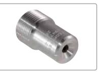
Ideal for close up cleaning of small parts, this blast nozzle features a tungsten carbide liner encased in an aluminium jacket, offering the greatest resistance to impact or flexing. Supplied with a rubber gasket, these nozzles are suitable for use with the Elcometer 1020 Abrasive Blast Machine.
