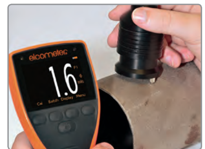
Integral or separate probes measure profiles up to 500µm (20mils) on flat or curved surfaces**
