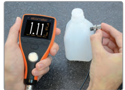
Ideal for measuring the material thickness of thinner materials such as plastics.
