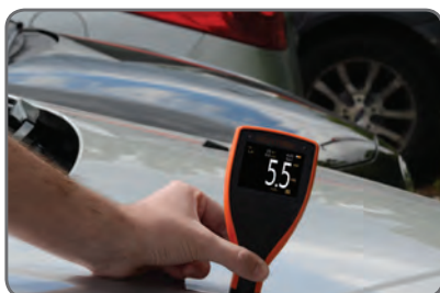
Measures on steel & aluminium body panels 2
