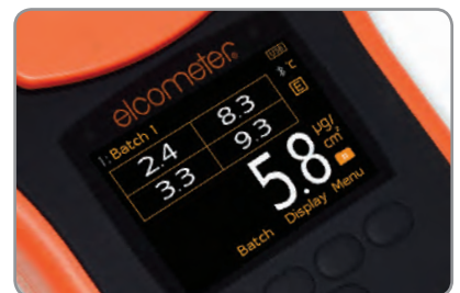
Four Bresle Patch Equivalent Readings
