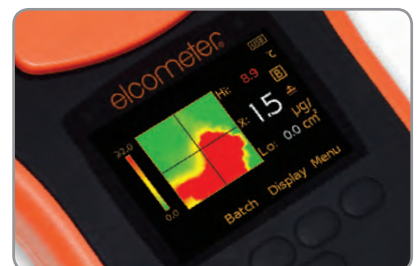
2D Salt Density Map with High/Low Readings
