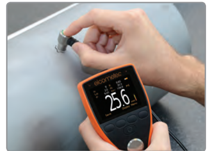
Ideal for measuring steel pipes where there is only access to one side.
