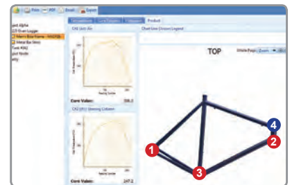
Individual product probe maps record the exact probe placement for each component.
